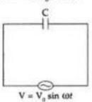
$$I = \frac{dq}{dt} = \omega \dot{c} V_0 \cos \omega t = I_0 \sin \left(\omega t + \frac{\pi}{2}\right)$$
